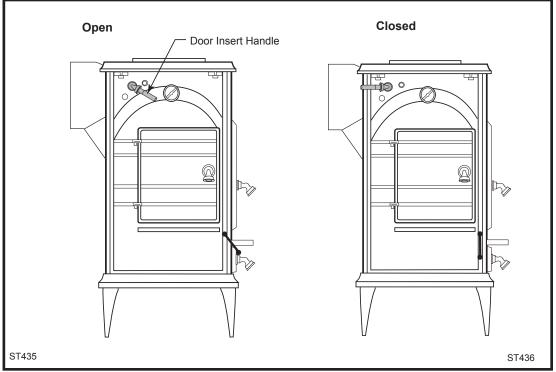
Fig. 24 Damper operating positions.
