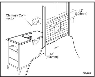
Fig. 10 Wall pass-through enclosed with noncombustible materials.
