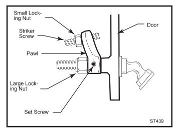
Fig. 27 Door latch adjustment.
