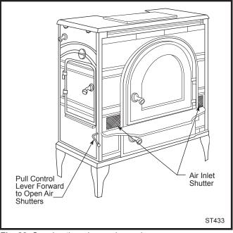
Fig. 22 Opening the primary air supply.
