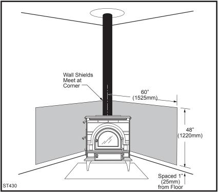
Fig. 18 Corner wall protection.
