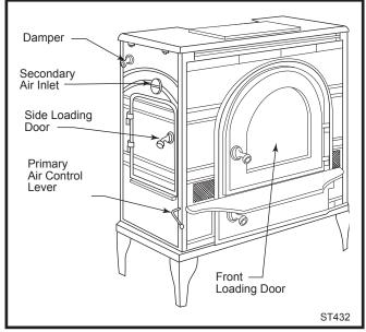
Fig. 21 The heater controls.
