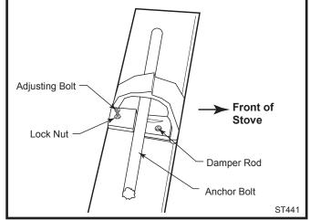
Fig. 29 Damper adjustment.
