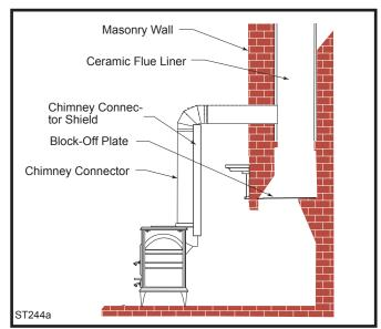
**Fig. 8** The connector enters flue above the fireplace. If the clearance between the chimney connector and either the mantel and/or the ceiling is inadequate, special protective shields will be required.
