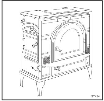
Fig. 23 Closing the primary air supply.
