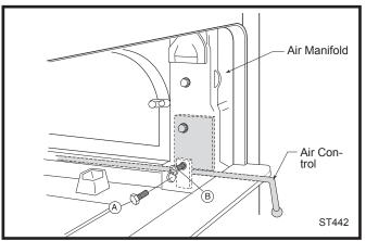
Fig. 30 Primary air control adjustment.
