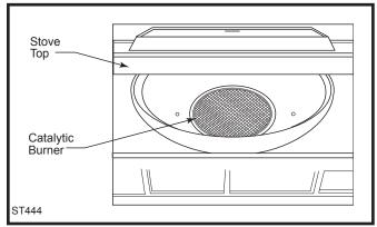
Fig. 32 Remove refractory package with care.
