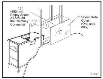
Fig. 11 Hollow wall pass-through.
